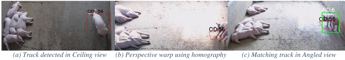
Figure 1: Simplified depiction of the Multi-Camera Tracking algorithm
